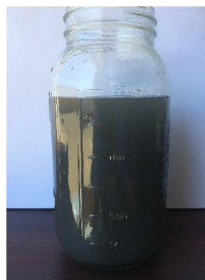
493 ppm oil 50 ppm Iron Oxide
